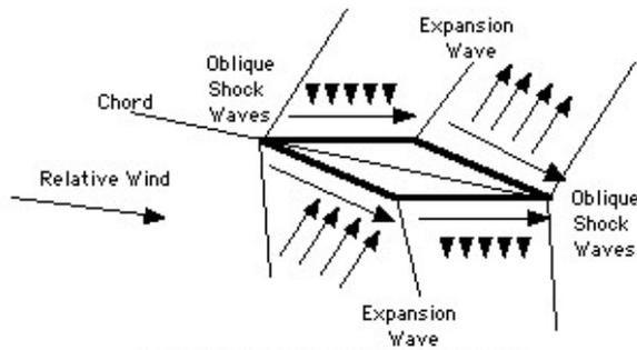
Figure 3: Creation of Lift on a Double Wedge Supersonic Airfoil
